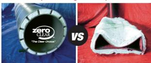
**ZeroClear™** after 2000°F (simulated grease fire) for 30 minutes.
